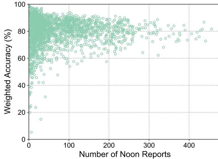
Figure 1: Scatter plot showing the weighted accuracy % on a vessel level, plotted versus the number of noon reports per vessel. As the number of noon reports increases the variance in the weighted accuracy % across all vessels is reduced.
