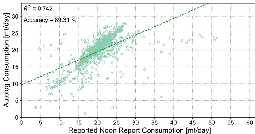
Figure 4: A case study of reported consumptions from noon reports compared to corresponding sensor data automatically collected aboard five tanker vessels, collected across a large time period. The  $R^2$  measure is derived from the best linear fit and the accuracy is calculated as the unweighted accuracy as given in (1).
