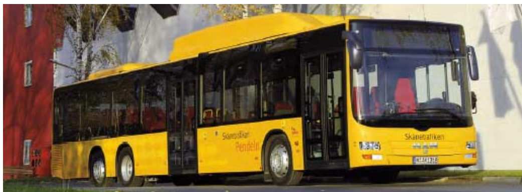
Figure 5-3 CNG Bus – The top of the bus stores the tanks with CNG. Source: MAN Nutzfahrzeuge – www.man-mn.com
